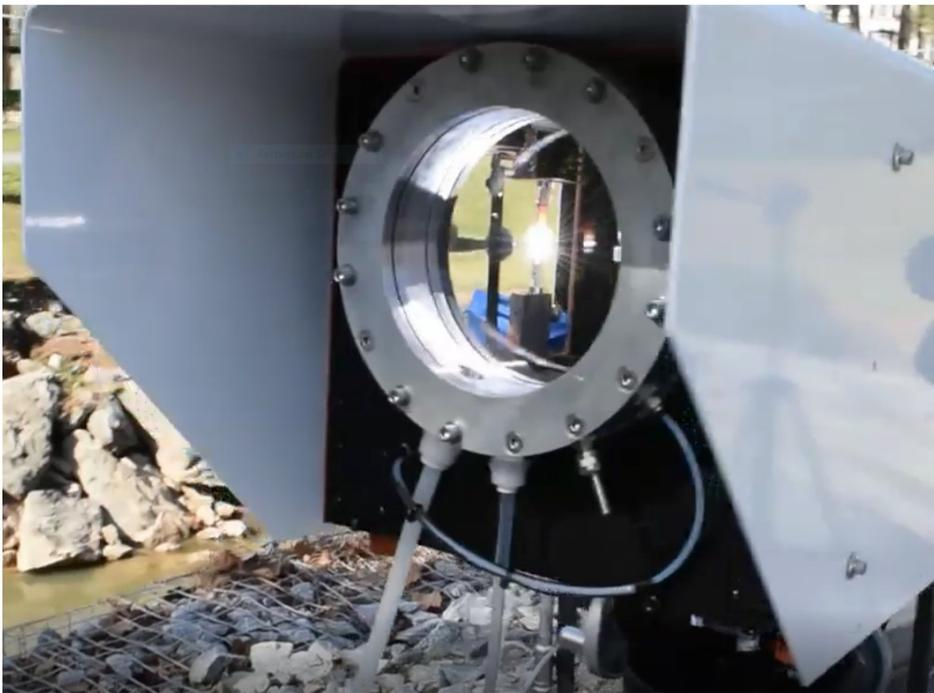
2.) 0.5 meter external linear cell (P/N 18101) may be used in lieu of the standard QA cell. The cell is placed in the beam path between the analyzer and retro-reflector and flooded with certified calibration gas. This cell is tripod mounted and useful for calibrating multiple analyzers as it is portable.
